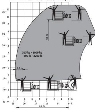
Machine on tyres with platform Imperial
