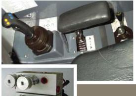
The tri-function joystick control option allows an operator to control the attachment tilt, auxiliary hydraulics and boom functions with a single joystick.
