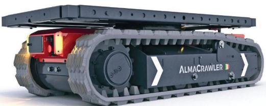
Easily extract the battery pack and eliminate downtime. The battery pack is equipped with its own inside charger directly.
