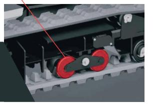
Increased accessibility and gradeability due to unique track design. The rollers actively adapt to the terrain, ensuringgrip and avoiding accidental load spills.
