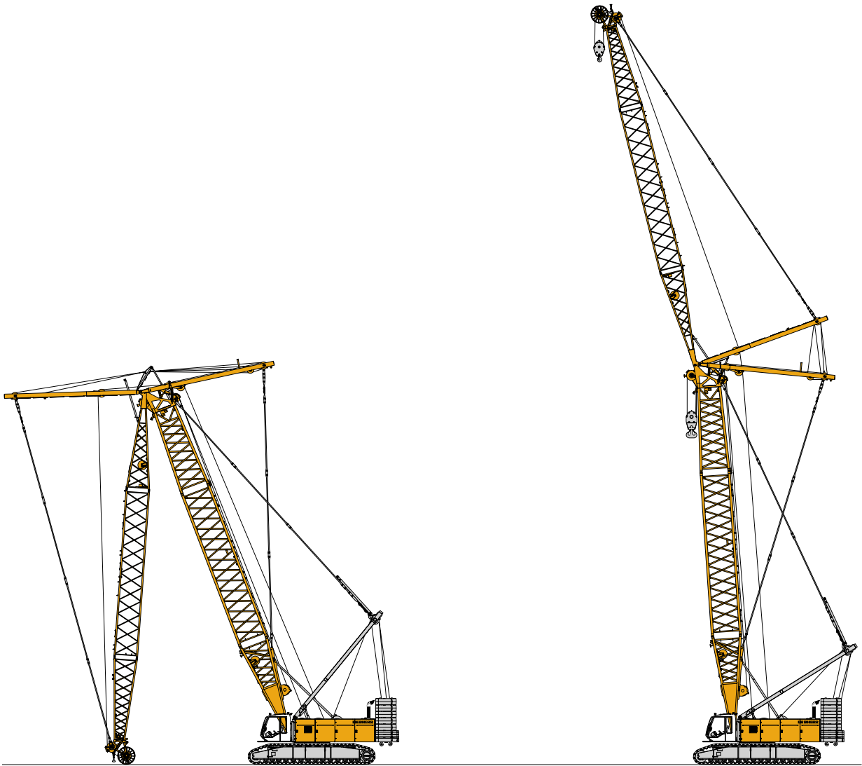
Erecting of main boom and luffing jib
