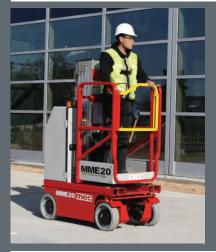
**Important** - MEC mast lifts must be on a hard level surface while elevated.
