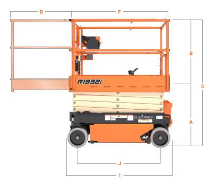
A. Platform Height (Lowered)38.6-in / 1.0-mB. Platform Railing Height43.3-in / 1.10-mC. Machine Height (Rails Raised)82.8-in / 2.1-mD. Machine Height (Rails Lowered)64.3-in / 1.63-mE. Platform Width25.4-in / .64-mF. Platform Length62.7-in / 1.59-mG. Platform Extension36-in / 91-cm
