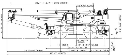
Note: Dimension is with boom angle at -0.8 degree.
