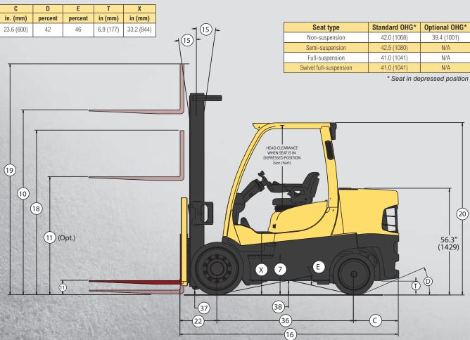
Circled dimensions correspond to the line numbers on the tabulated chart inside the Technical Guide. Dimensions are in inches (millimeters).
