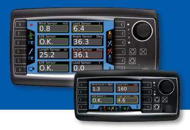
The PRS 90's flexible design allows for monitoring single or multiple wireless and/or hardwired sensors. The sensor inputs are displayed on a color graphic display which is capable of monitoring and displaying the status of up to eight sensors at one time.
